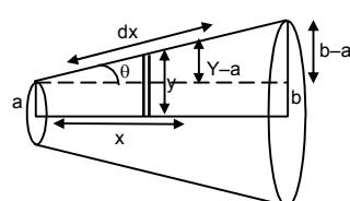
$$\begin{aligned}\Rightarrow Ly - La &= xb - xa \\ \Rightarrow L \frac{dy}{dx} - 0 &= b - a \quad (\text{diff. w.r.t. } x) \\ \Rightarrow L \frac{dy}{dx} &= b - a \\ \Rightarrow dx &= \frac{L dy}{b - a} \quad \dots(2)\end{aligned}$$
